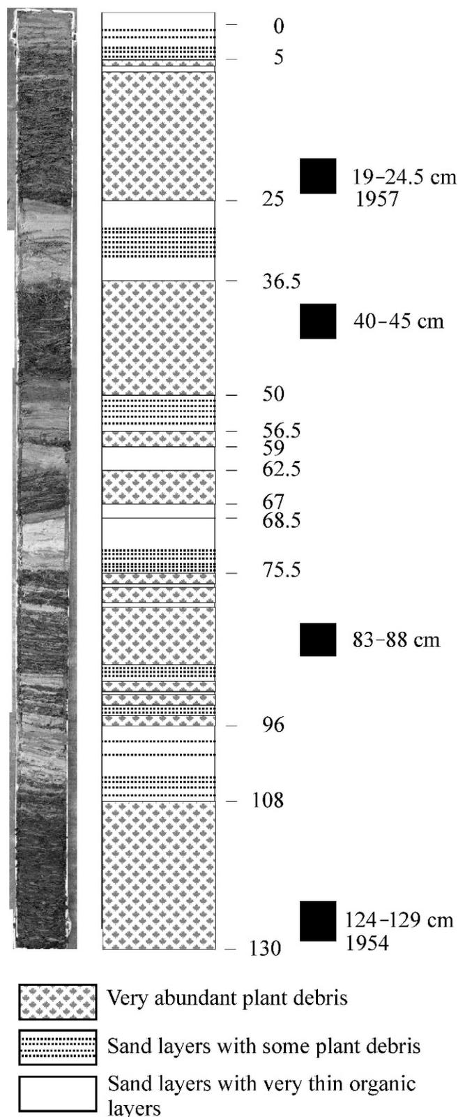
FIGURE 3—Core taken from Site II, point 3, on the Preto River (left), accompanied by a schematic drawing showing details of the thickness and composition of the layers. Note the cyclic nature of thick layers of plant debris interspersed with layers of fine sand containing few plant remains. Black squares show the level of samples collected for  $^{14}\text{C}$  dating. Scale in meters.
