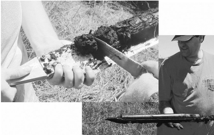
Figure 5. Russian auger used in the collection of samples (bottom) and detail of sampling every 3 cm of depth (top).
